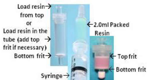
2.0ml Syringe Column for Affinity Resins (Ni-, GST, Protein A & G and other resins)
